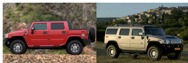
Left: Hummer H2 SUT– not classified as a passenger car since the luggage space is separated from the passenger compartment. Right: Hummer H2, classified as a passenger car. Photo: GM Corp.
